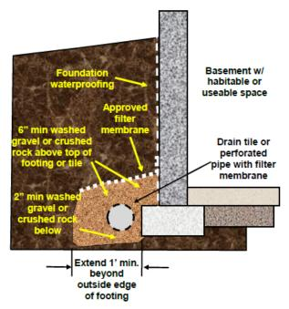
Drains must discharge by gravity or mechanical means to an approved drainage system
